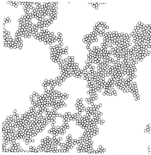
Fig. 6. The percolating cluster of disks generated by increasing the disk radii in Fig. 4 by 20%.
